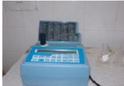
Figure 3-9: Hach spectro- photometer used to measure COD.
