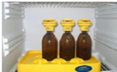
Figure 3-8: OxiTop device used to measure BOD
